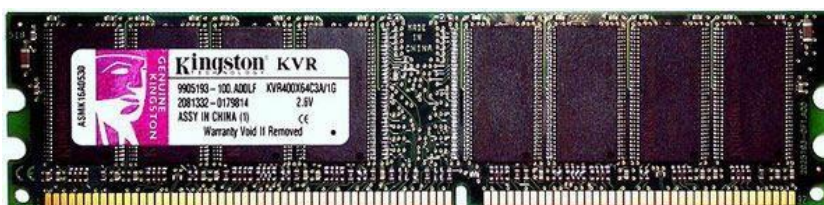
DDR SDRAM yaddaş modulu, 184 pin
